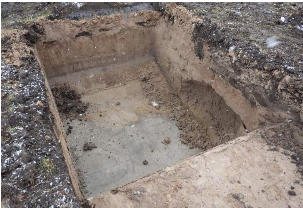
Plate 28: Test Pit 4 (TP04) carried out at the western end of Trench 4. Change to blue-grey colour sands at 1.20m BGL
