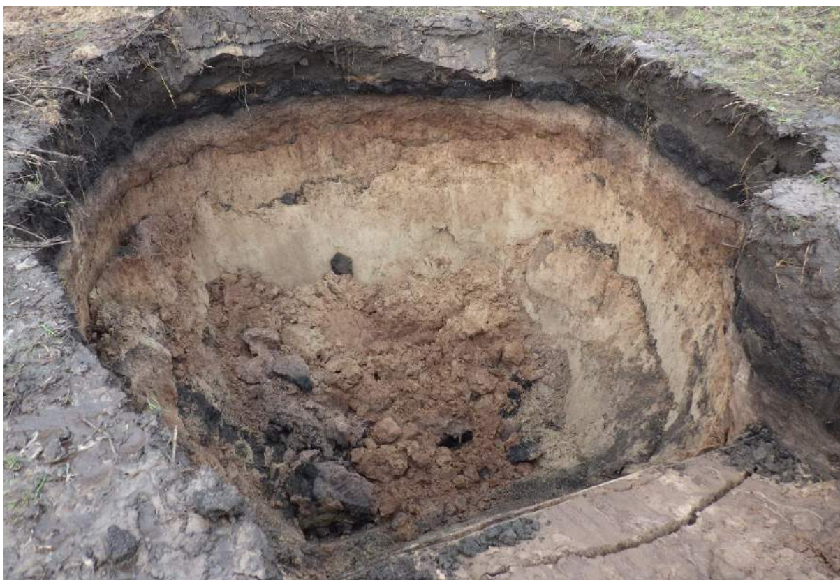
Plate 22: Test Pit 2 (TP02) collapsing at 2.50m BGL
