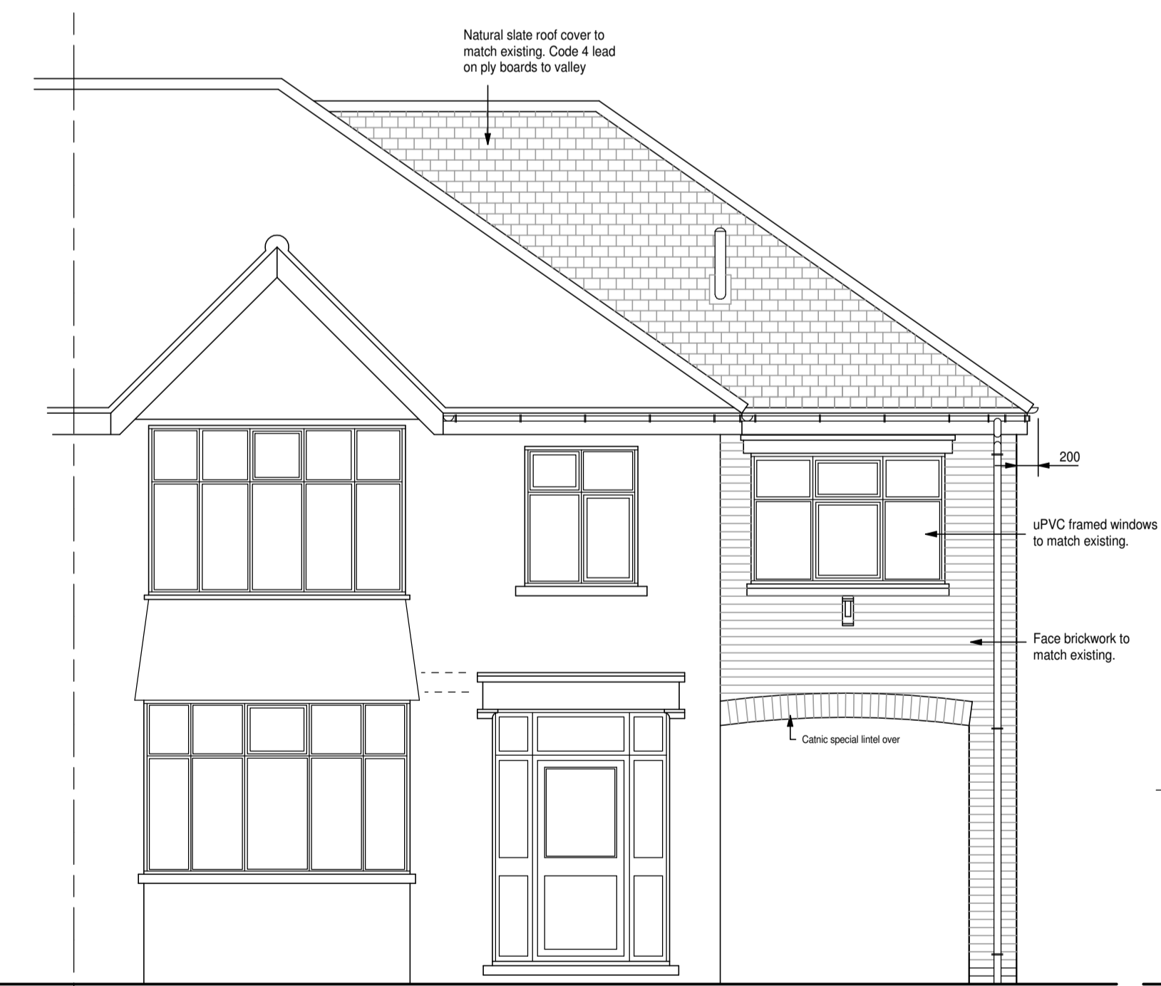
Proposed Front (East) Elevation
