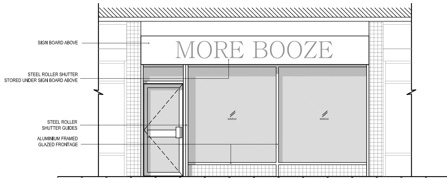
EXISTING FRONT ELEVATION
