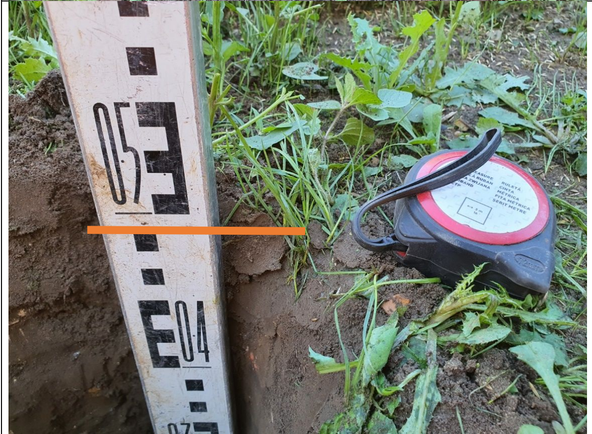
Trial pit 1 – rear garden topsoil
