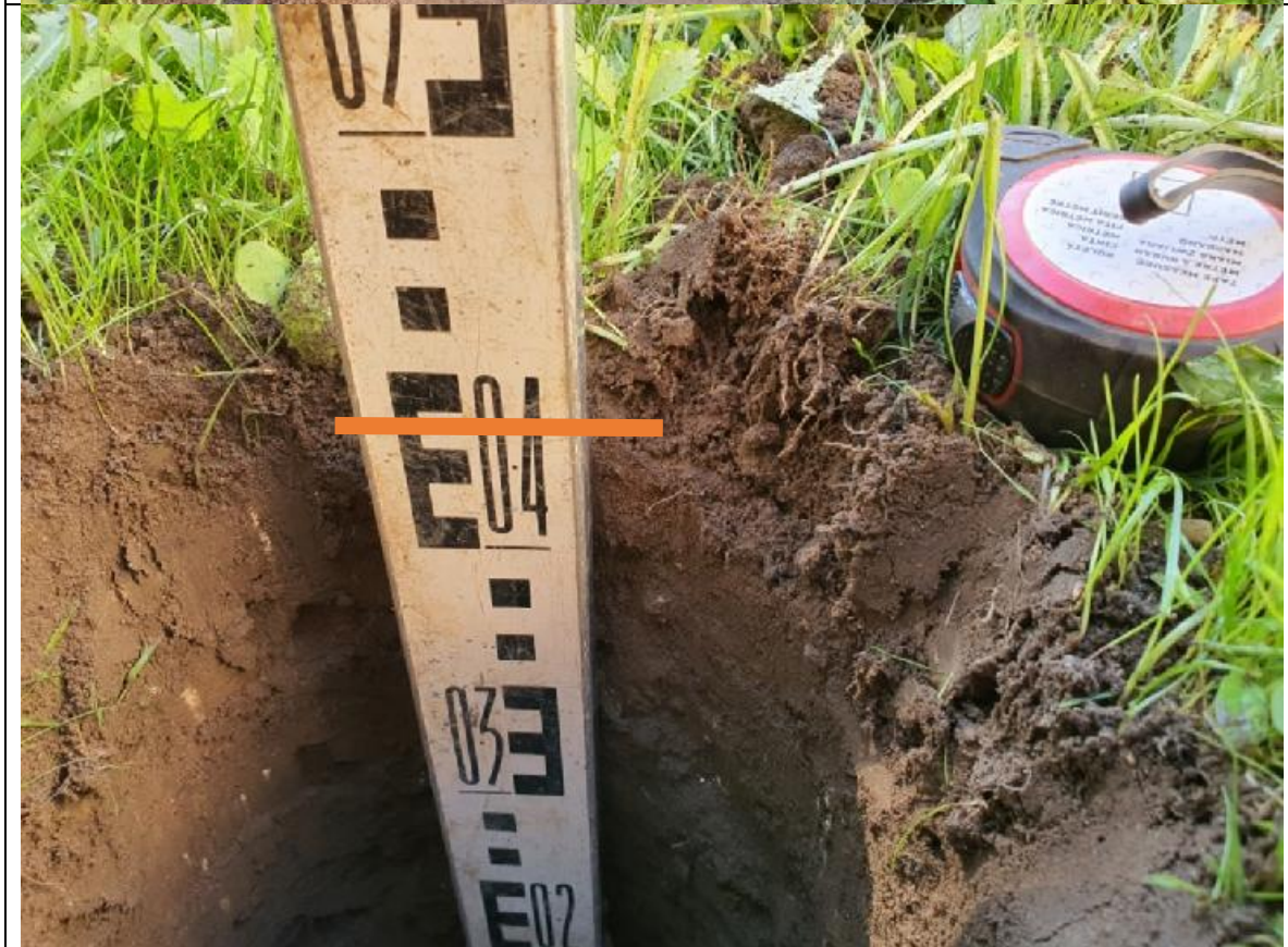
Trial pit 2 - rear garden topsoil
