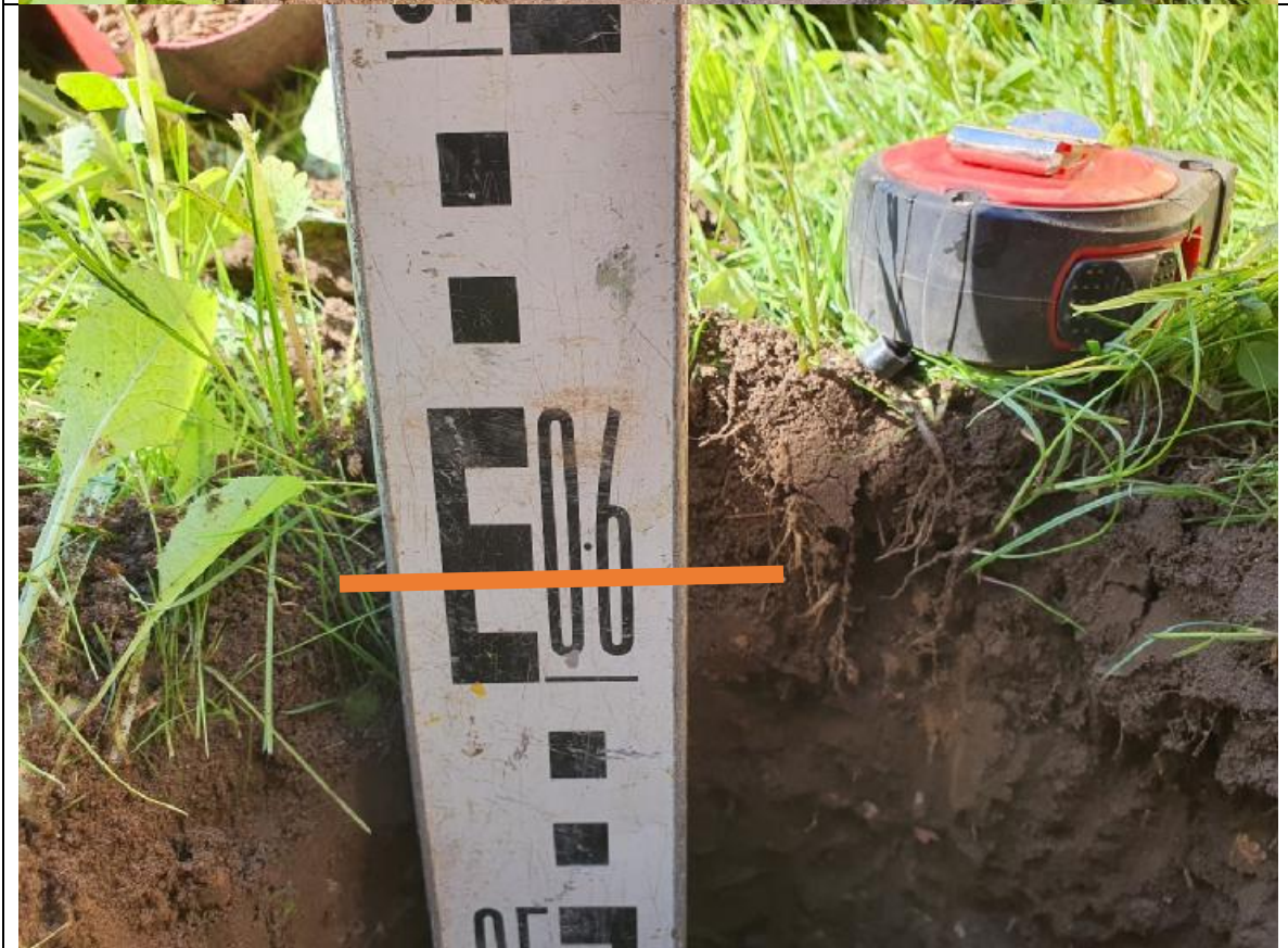
Trial pit 2 - rear garden granular capillary layer
