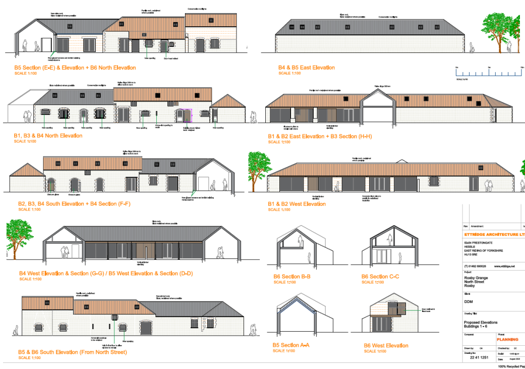
Fig. 62 – proposed elevations for the conversion and rebuilding of the main yard buildings
