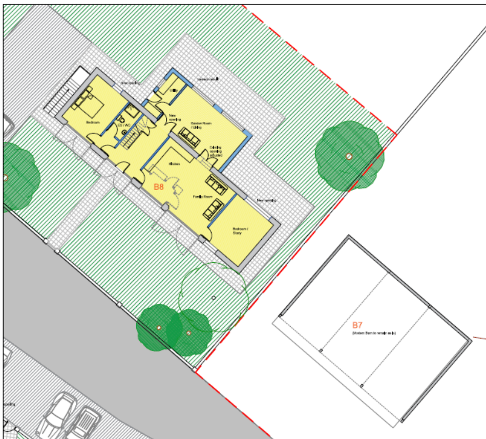
Fig. 61 – the ground floor layout for the conversion of Building B7 (noted as B8 on this drawing) to a single dwelling
