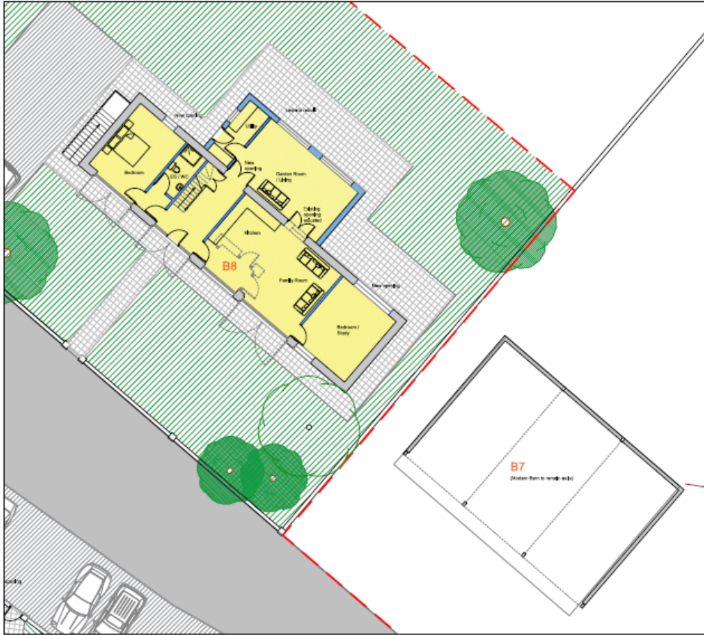
Fig. 19 – the ground floor layout for the conversion of Building B7 (noted as B8 on this drawing) to a single dwelling
