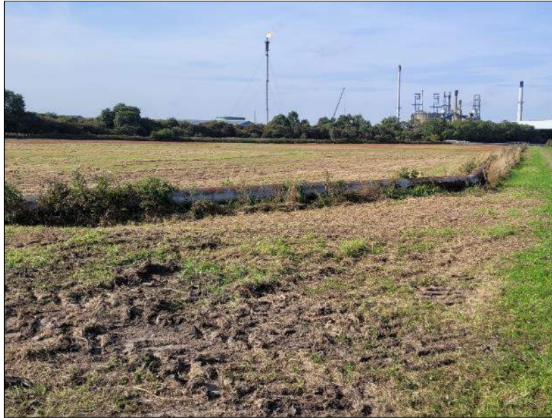
Plate 9: Above ground metal pipe associated with magnetic noise [12], looking west-southwest
