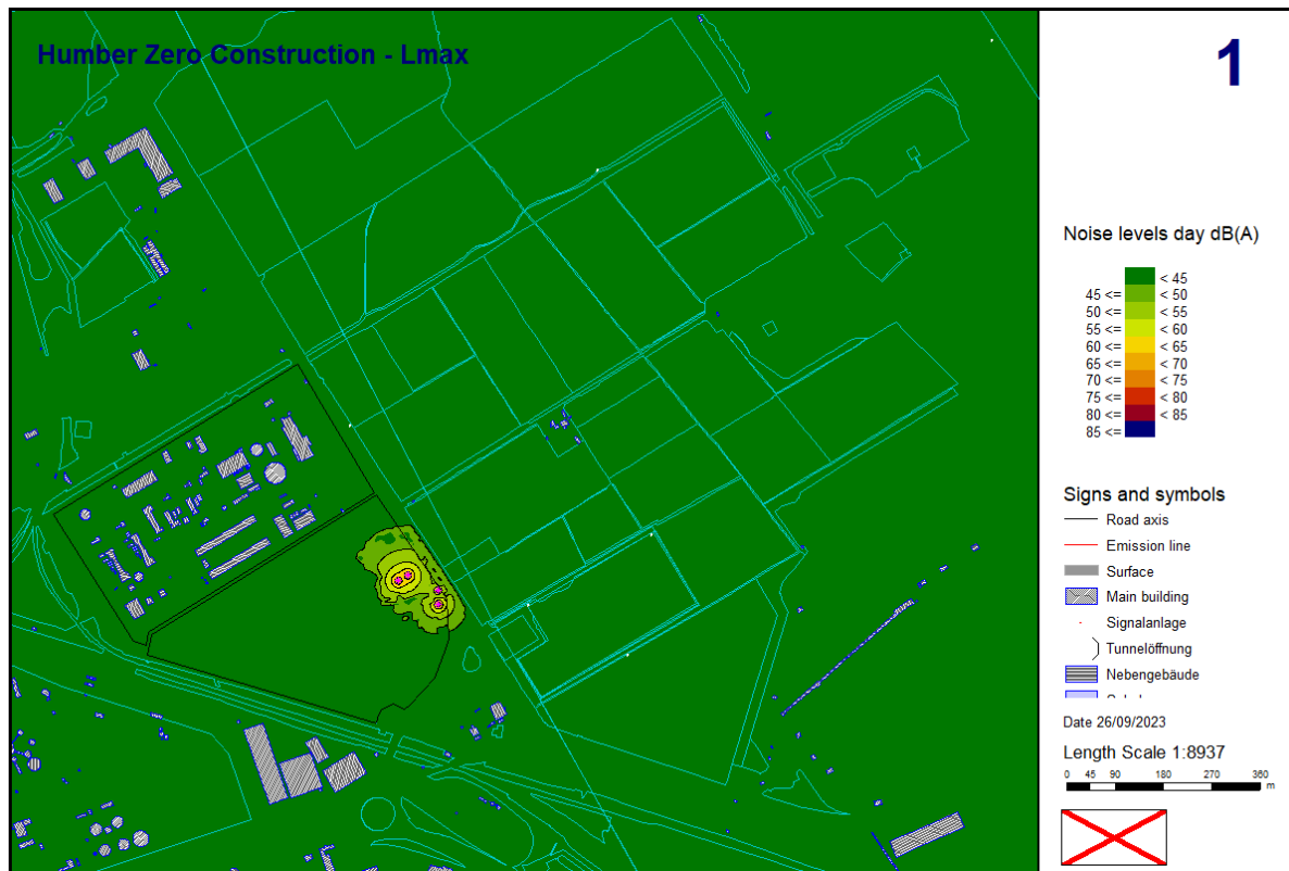
Figure A3 – Proposed VPI Development Construction (alone) LMax
