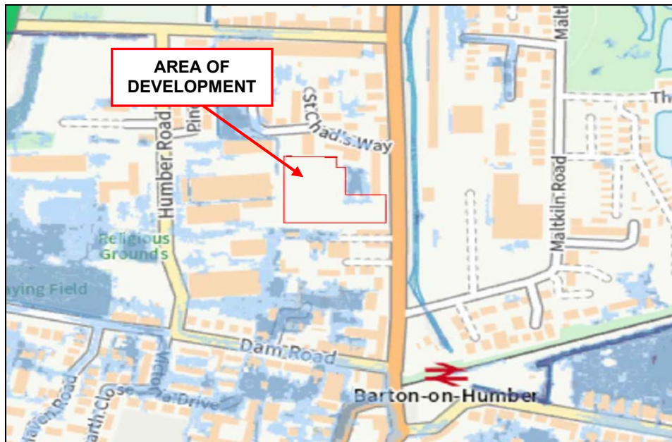
Figure 6: Environment Agency map dated May 2023 showing the anticipated flood depth from surface water – low risk
