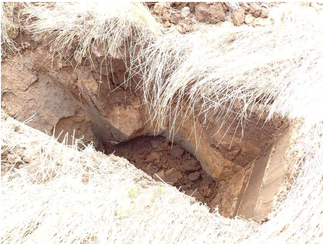
Collapsed section of TP05
