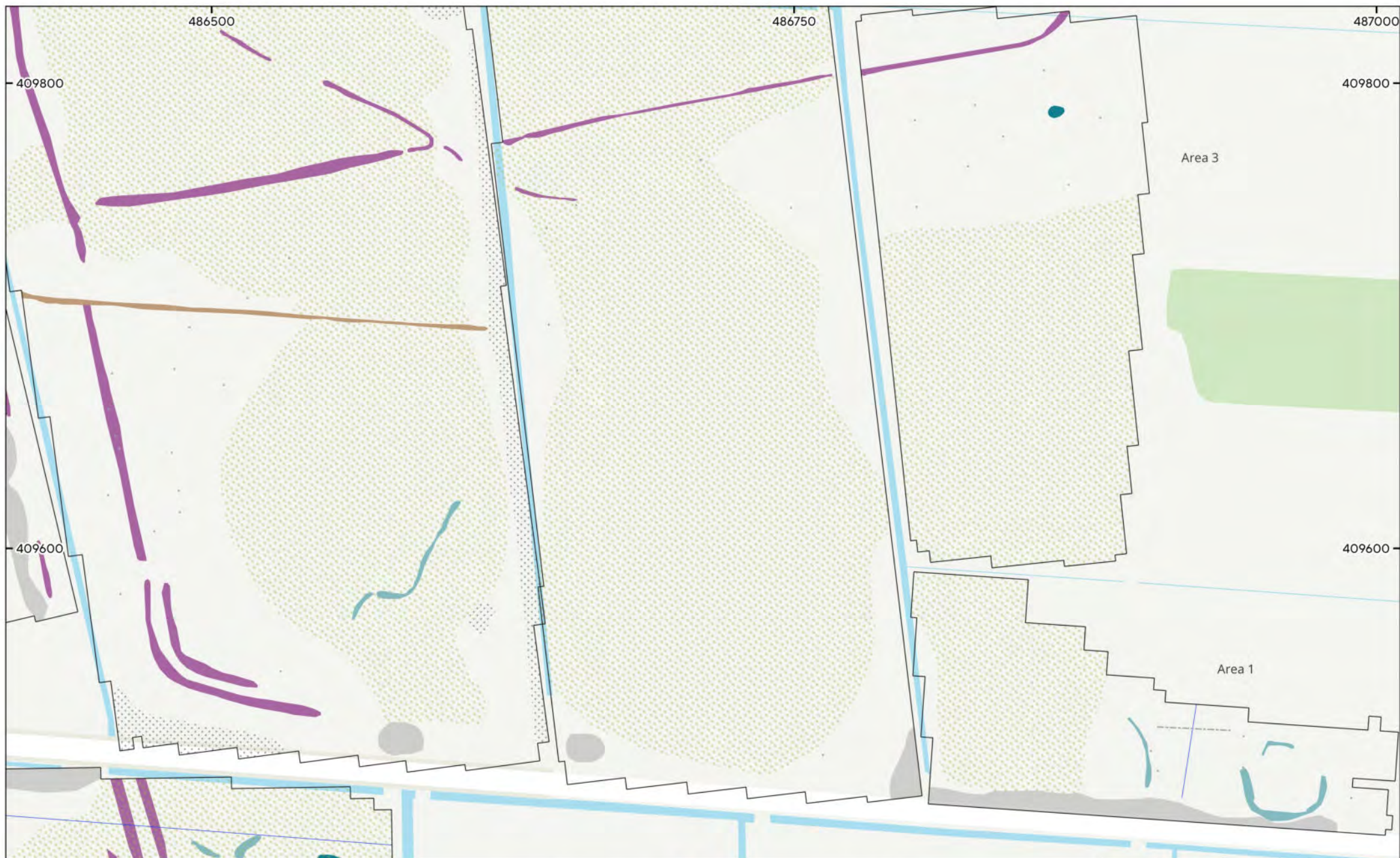
MSSE1894 - Lincolnshire Lakes Figure 18 - Magnetic Interpretation (Areas 1 - 3) 1:1,500 @ A3 © Magnitude Surveys 2024 Contains Ordnance Survey data © Crown Copyright and database right 2024
