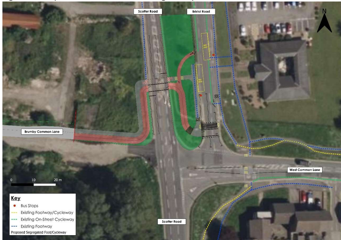
Figure 17: Proposed Scotter Road Crossing Facility
