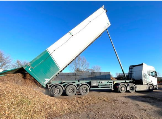
HGV tipping material into yard storage area
