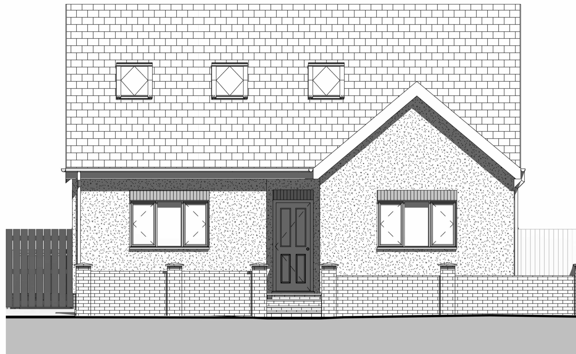
Proposed Front Elevation 1 : 50
