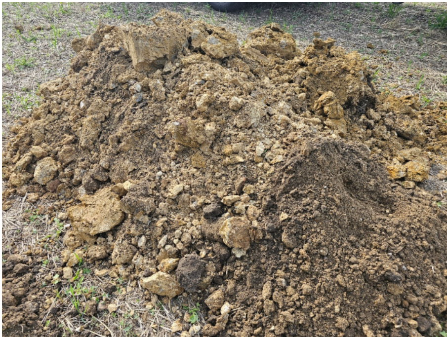
Site investigation photo: 4 Date: 27 Jun 2025 Photo direction: - Description: Glacial deposits from TP201
