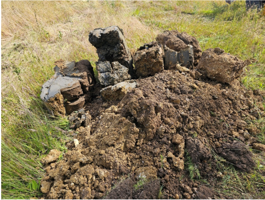
Site investigation photo: 19 Date: 27 Jun 2025 Photo direction: - Description: Light brown glacial deposits and deeper grey possible weathered mudstone clay from TP205
