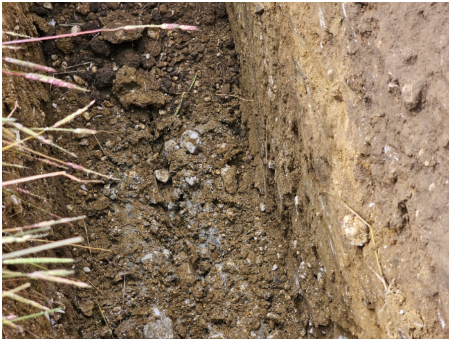
Site investigation photo: 22 Photo direction: - Description: TP206 – close-up of light brown sandy gravelly boulder clay
