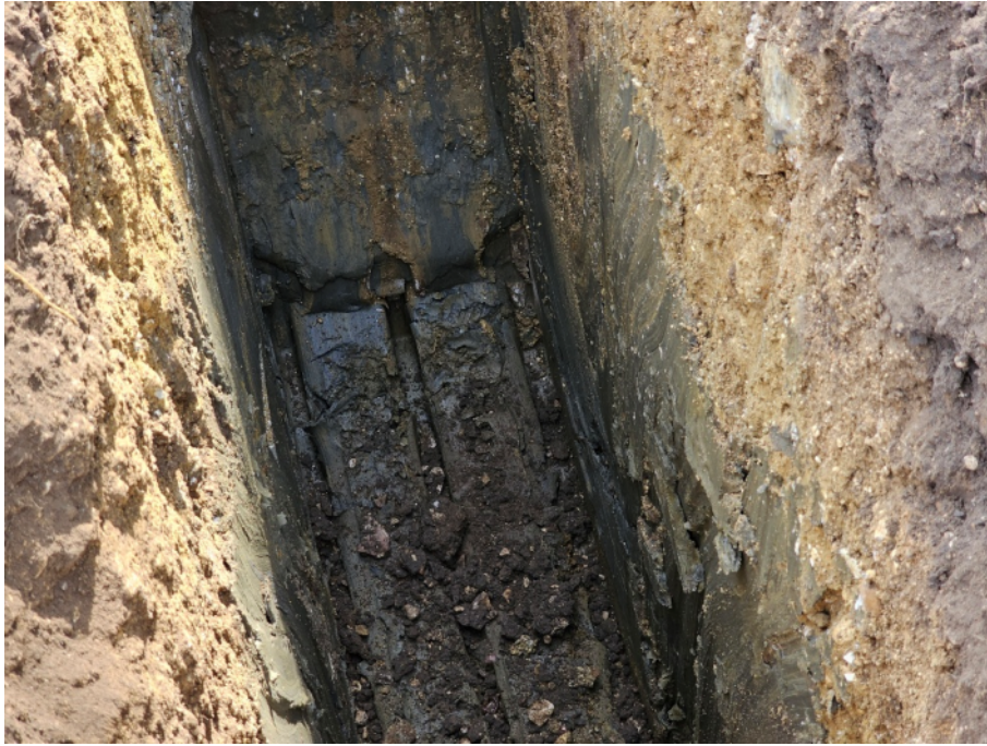
Site investigation photo: 17 Date: 27 Jun 2025 Photo direction: - Description: TP205 – close up of possible weathered mudstone / stiff clay
