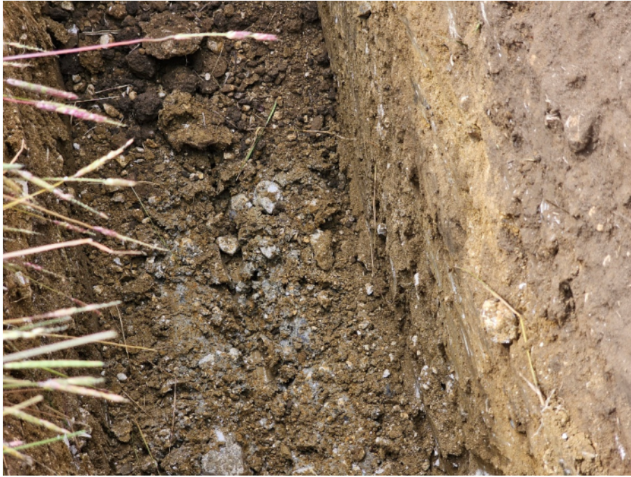
Site investigation photo: 23 Date: 27 Jun 2025 Photo direction: - Description: TP206 – close-up of light brown sandy gravelly boulder clay
