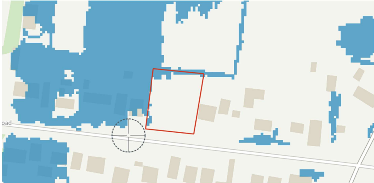
Figure 2.5 - Risk of Flooding from Surface Water Mapping
