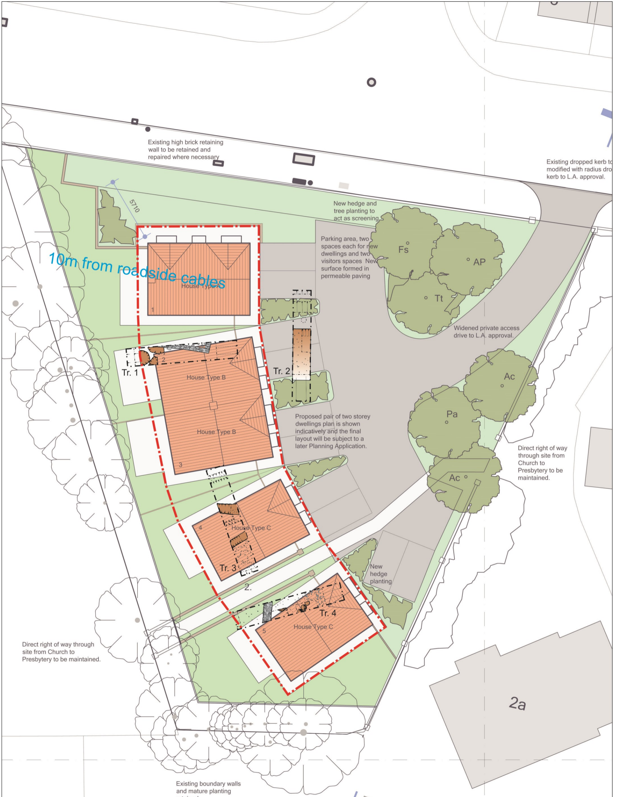
Figure 2: Barrow Road, Barton. Proposed site development plan (RDA drawing ref R:5251/11 Rev B) overlain with the trenching results (Lane, 2023) and showing the planned excavation area outlined red. 1:200 @ A3.
