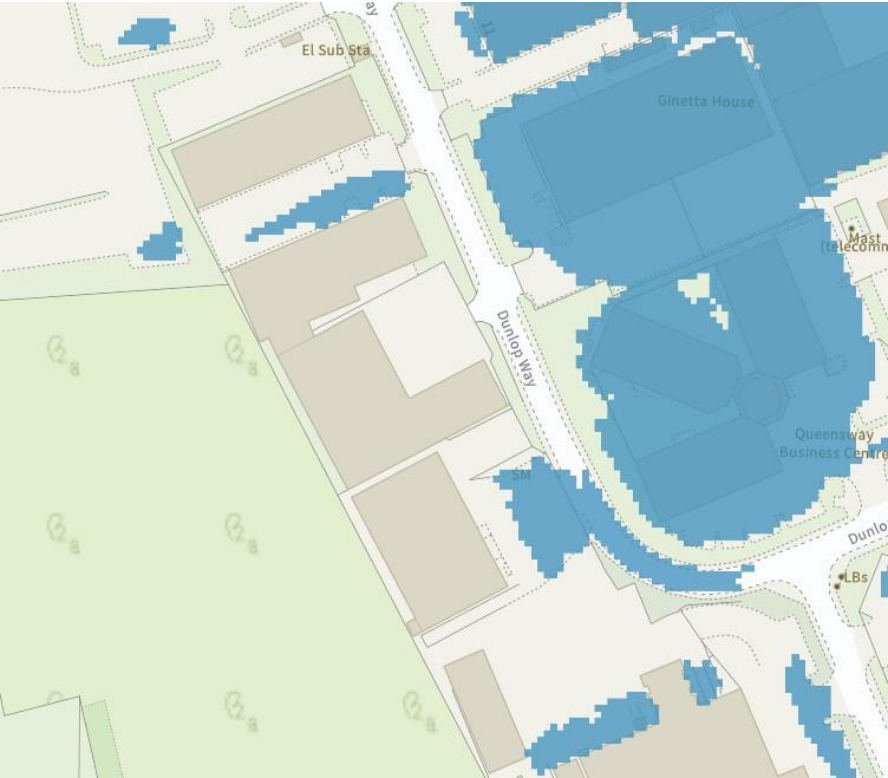
Figure One - 1 in 30-year surface water maps.
