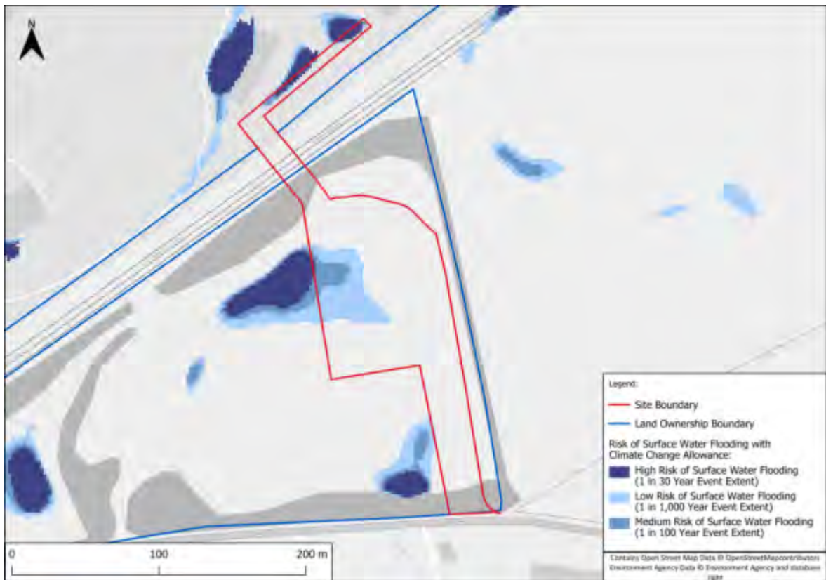
Figure 5-2: Risk of Flooding from Surface Water with Climate Change 1 Mapping Extract
