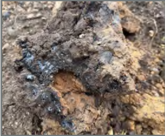
Figure 13. Small self confined piece of suspected tarry soil removed from TP4
