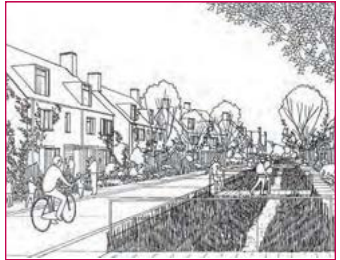
Above: Illustration from planning application for Villages 1 and 5 showing how drainage ditches might be incorporated within the street
